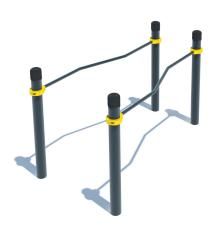
The complex consists of four vertical columns and two multi-width parallel bars 1790 mm in length. The distance between the parallel bars is 608 mm at one end and 1008 mm at the second end. Total width difference for the parallel bars is 400 mm. Construction is secured together with aluminium clamps. Weight - 79,80 kg
