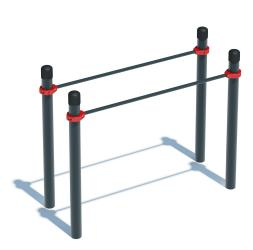
The construction consists of four vertical columns and two horizontal crossbars. Crossbar length is 1758 mm. The distance between the parallel bars is 600 mm. Crossbars are secured to the columns with aluminium clamps at the height of 1300 mm from the foundation. Weight 91.2 kg
